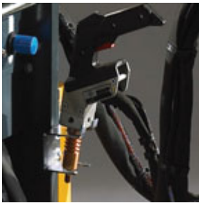
Single sided gun for spot welding from one side and dent pulling
